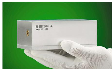
Fig.1. Baltic SP nanosecond laser. Pulse energy -10mJ; Pulse duration – 12ns; Repetition frequency – Single shot÷10Hz; Beam shape - Multi-mode.
